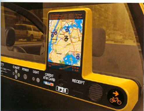
Opposite page: Ken Smith Landscape Architect: The Green Taxi proposal imagines compact, fuel-efficient vehicles using dedicated taxi lanes Above: Antenna Design New York Inc.: A redesigned partition increases visibility while integrating a host of features, from a power outlet and reading light to an information display with real-time map, tip calculator, and more
